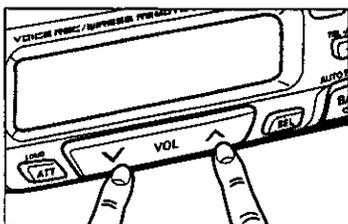
**Note:** When a control mode (BAS/TRE/BAL/FAd) is selected but no operation is made within 5 seconds, the display will return to the normal operation (volume adjustment) mode. In such a case, press SEL again to select the next control mode.
