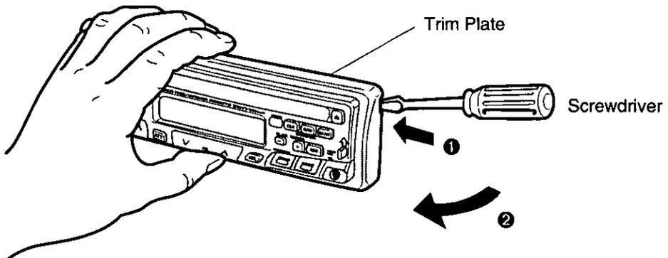
b) Pull out the unit while pushing the lock lever using a screwdriver.
